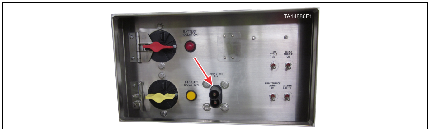
Figure 7: Jump start connection located inside switch box assembly (current production machines)
