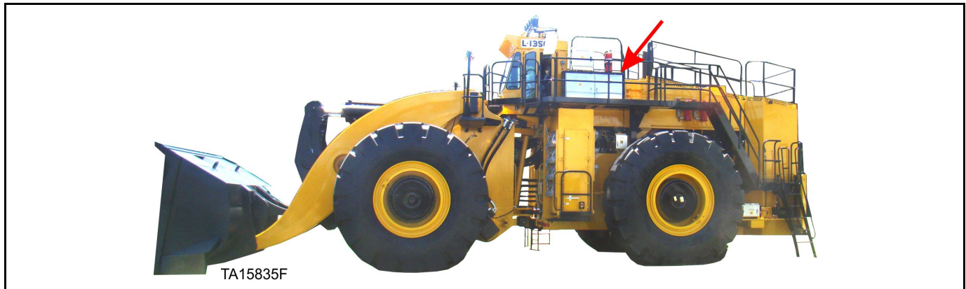
Low voltage control cabinet (shown on L-1350)
